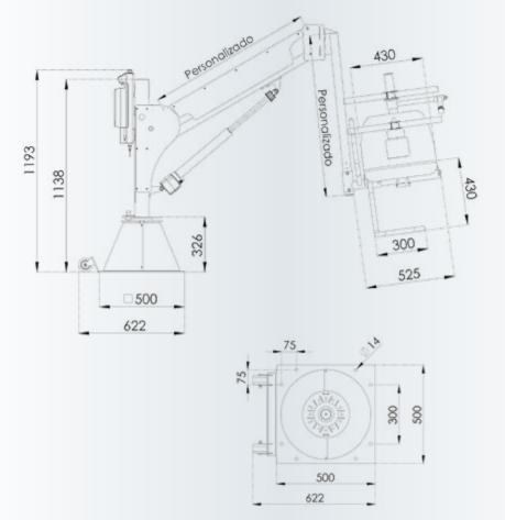
The anchor plate, made of 316 stainless steel, maintains its dimensions regardless of the pool profile.
